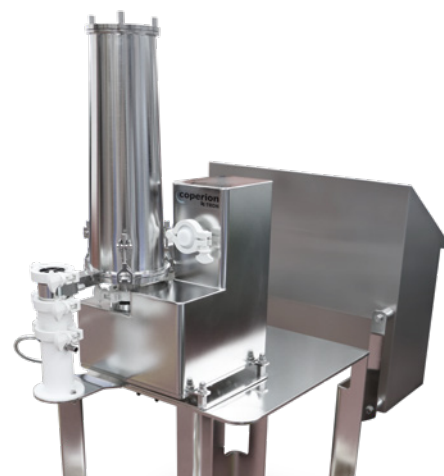
Photo 2: Coperion K-Tron MT16 ESL Gravimetric Feeder
